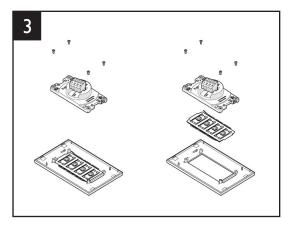
Using a Phillips screwdriver, disassemble the Lutron Palladiom keypad base by unscrewing the (4) screws on the back.
