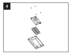
Place the TRUFIG fascia face down on a flat and smooth surface with the UP arrow in the correct orientation. With the buttons in the correct orientation, reattach the Lutron Palladiom keypad base unit to the TRUFIG Palladiom Fascia with attached buttons, using a Phillips screwdriver.
