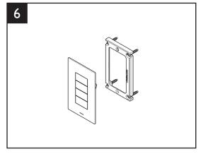
The assembled TRUFIG Palladiom keypad attaches to the TRUFIG Palladiom Trim Component using the keypad's magnets.
